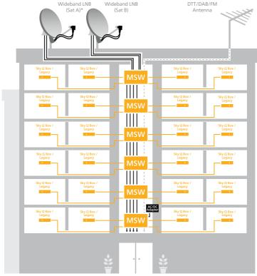
$<sup>^*</sup>$  If Sky service is required to be distributed, it should be connected over the SAT A position MSW = Multiswitch
