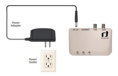
8. Plug the other end of the power adapter (external, 12VDC, 1A) into an electrical outlet.
